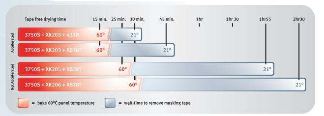
3750S offers a wide window of available drying times, allowing you full flexibilty in your workflow. Overall drying times are greatly reduced, thus speeding up your throughput while saving energy from lamps or oven.
